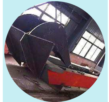
Proof Load Test 100% proof load test for each anchor
