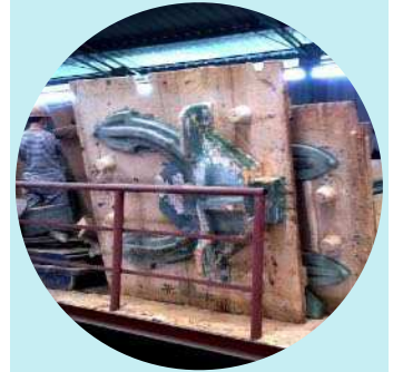
Anchor Moulding Types of moulds for casting anchors
